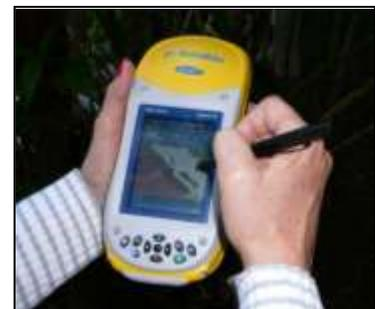
Using a handheld GPS data logger (Trimble Geo XM Unit with sub meter positioning accuracy) to collect and verify information, the inventory database will facilitate and expedite the repair and replacement of large numbers of
